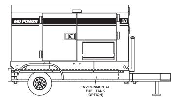
Figure 21. Internal Fuel Tank System
